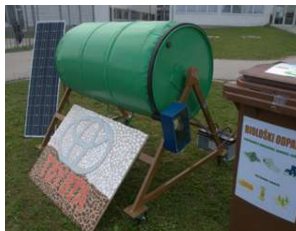
Preserje Pri Radomljah Primary School's winning design – a solar powered composting machine made with recycled Toyota car parts.
